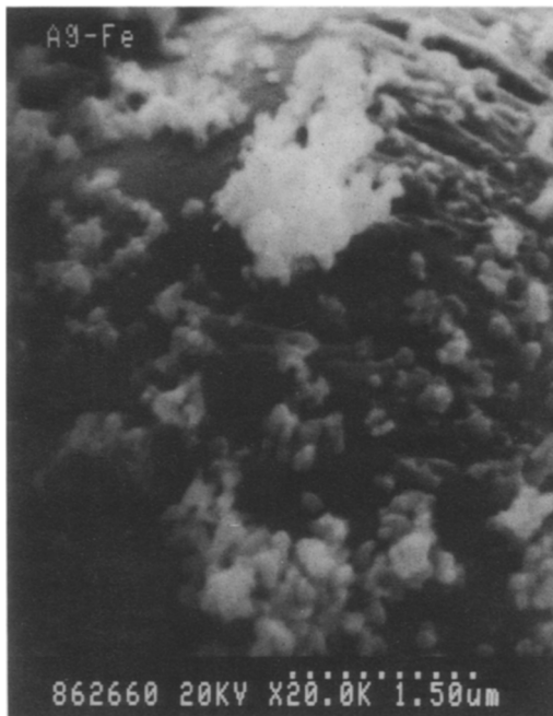
FIG. 7. SEM(S-520) micrographs for seriously poisoned catalyst.
